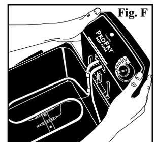
**Important:** The magnetic cord was designed to detach easily from the fryer. As a result, if it is bumped or touched during use it could possibly detach causing the unit to stop heating. Avoid contact with cord during operation. If contact occurs, verify that the cord is still properly connected.
