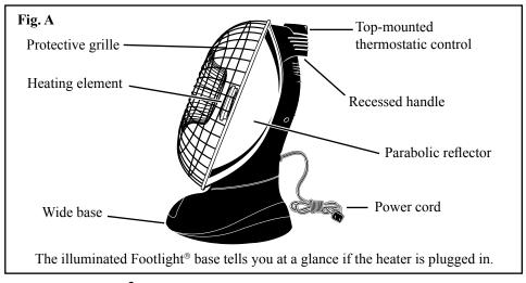
ON. In addition, the buzzer may sound and the heater will shut off if too much dust or dirt has accumulated on the parabolic reflector. To clean the parabolic reflector, see cleaning instructions on page 4.
