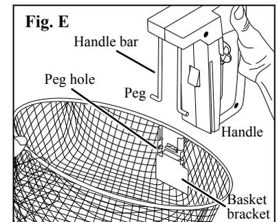
3. Next, place one of the pegs in one of the peg holes. Then squeeze the handle bars together and fit the opposite peg in the other peg hole (Fig. F).
