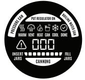
canning method and processing time using the control knob and advance button. From there on, the LED digital display will illuminate what the canner is doing and what phase the canner is in: warming, heating, venting (specific to pressure canning), canning, cool down, and done. The display will also communicate what action is required of the user:
